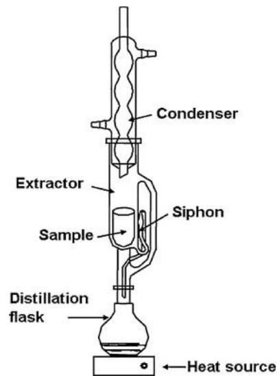
Fig: Soxhlet apparatus
