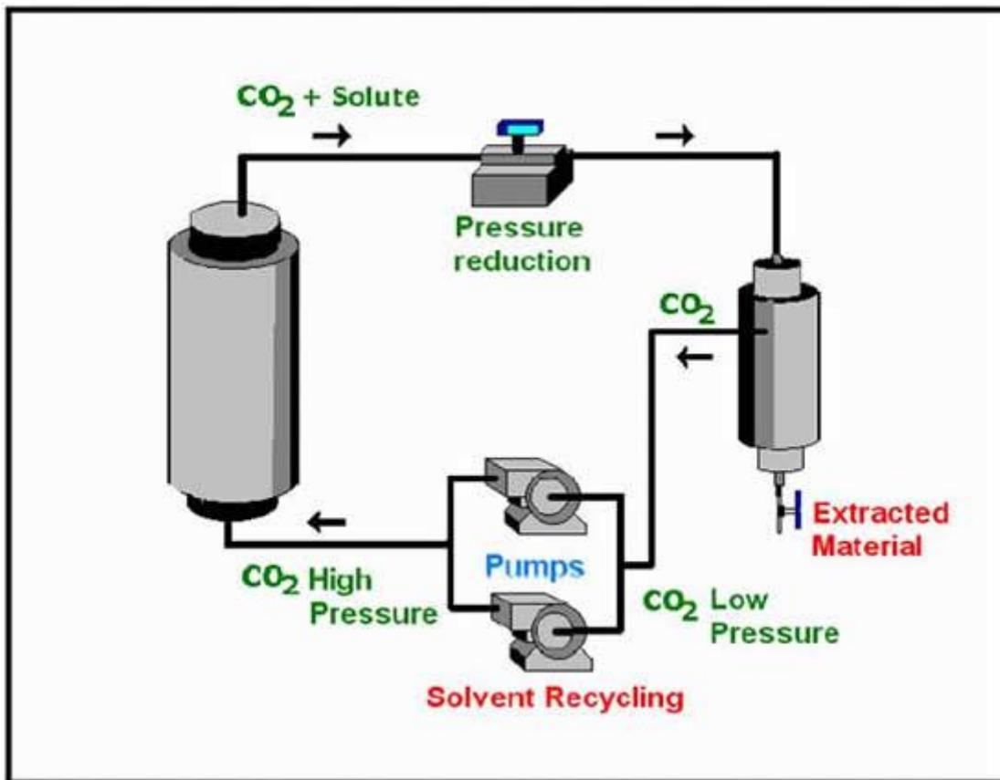
Fig: A schematic diagram of a supercritical fluid continuous extraction.
