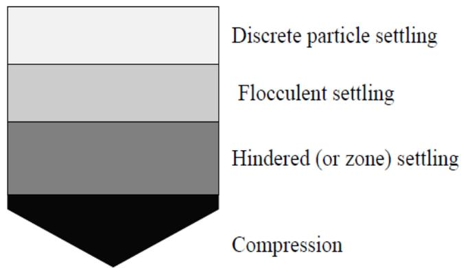
Fig: Settling phenomena in a clarifier
