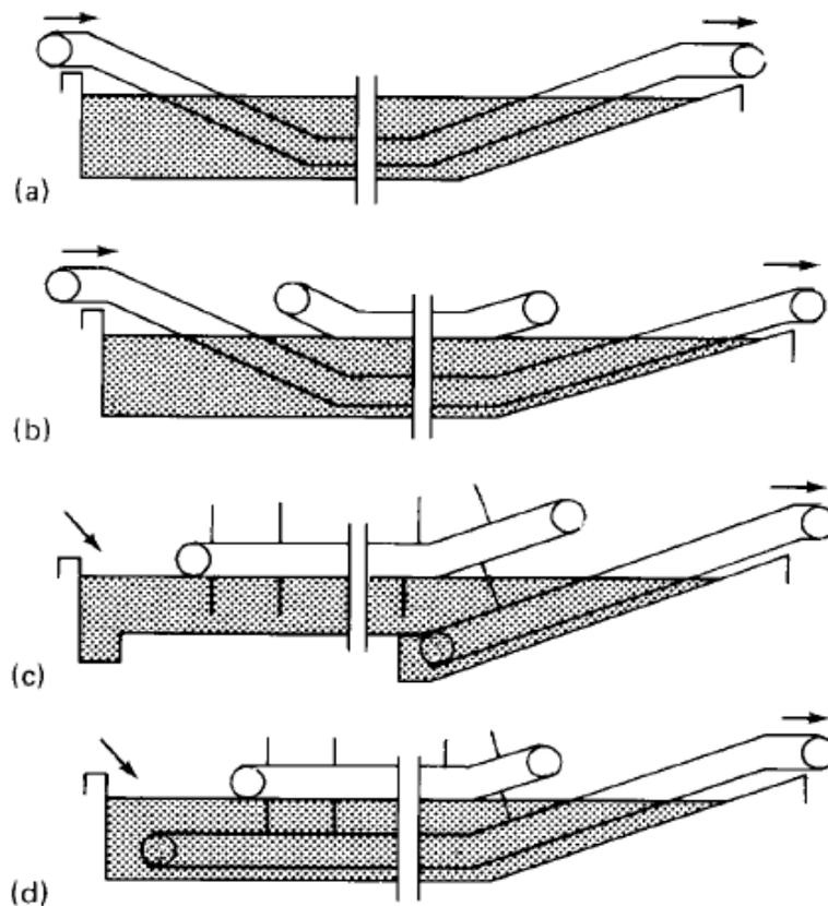
**Fig. 17.3** Different conveyor arrangements: (a) delicate non-buoyant products (for example fish sticks); (b) breadcrumb-coated products; (c) dry buoyant bulk products (for example half-product snacks); (d) dual purpose (for example nuts and snacks).
