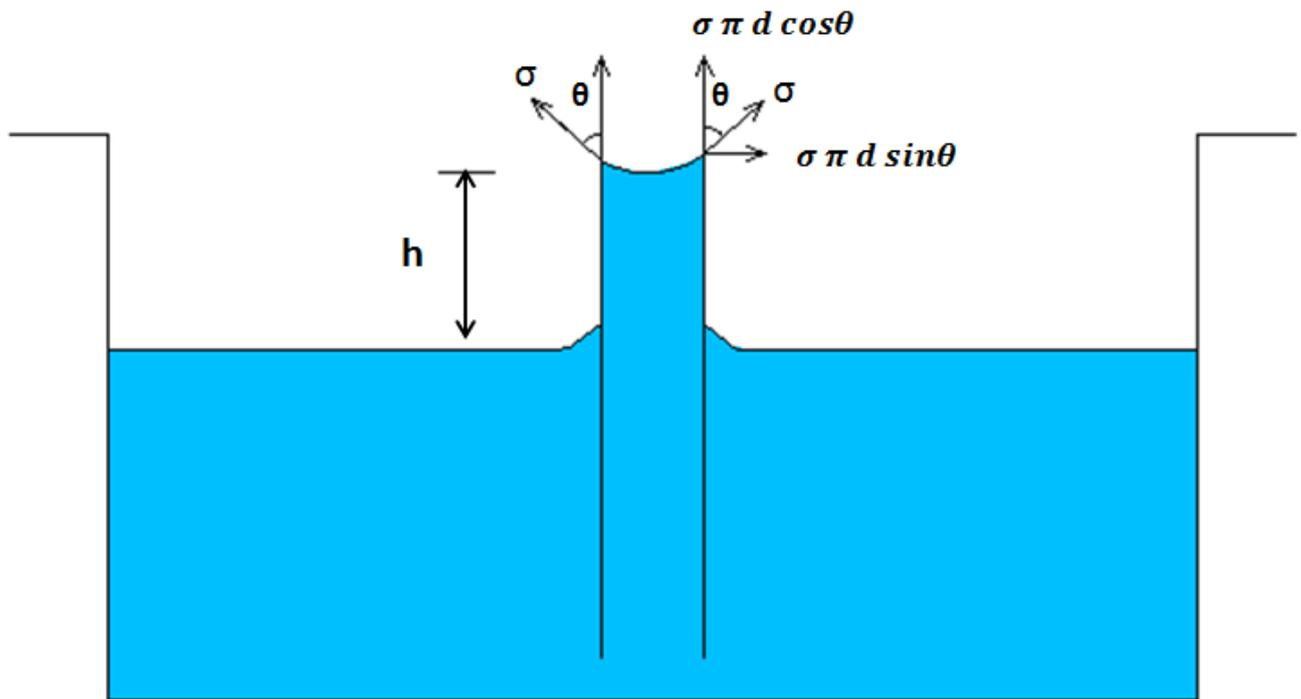
**Fig.: Effect of capillarity**
