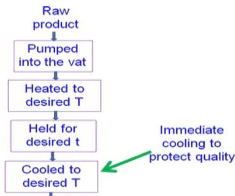
Figure: Basic operations in a vat pasteurizer
