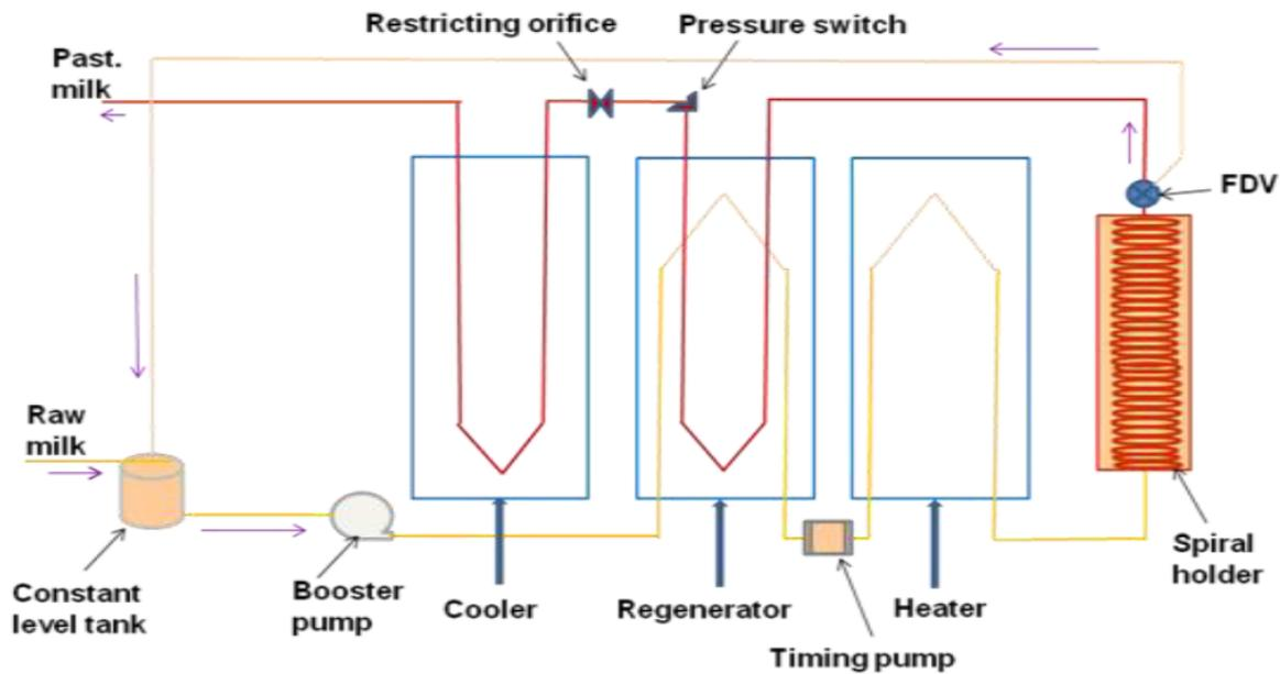
Figure: HTST pasteurization process
