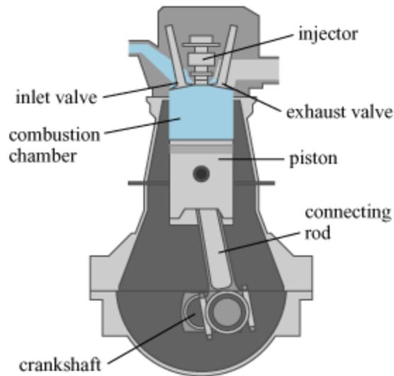
Figure: Compression ignition (CI) engine
