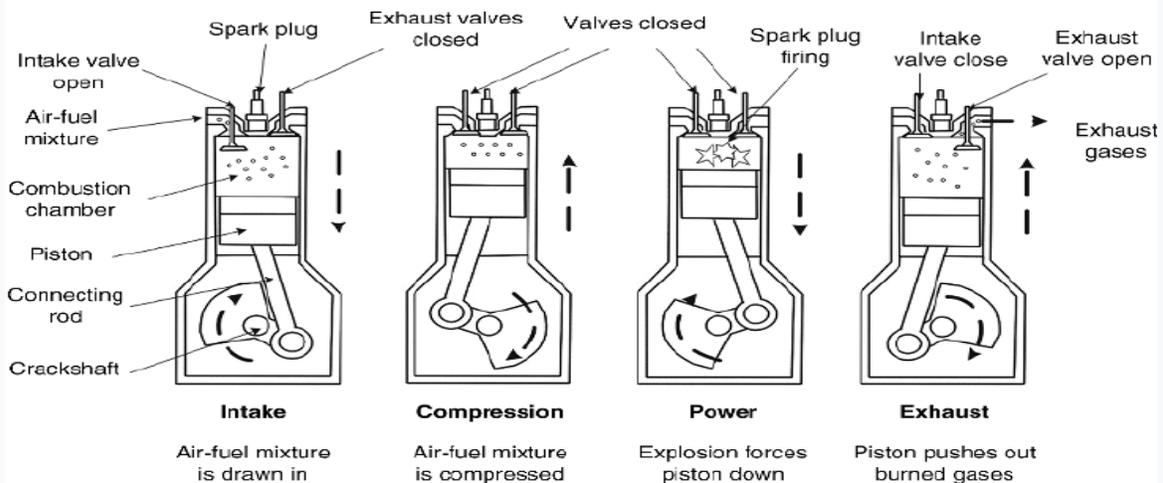
Diagram showing the operation of a 4-stroke SI engine. Labels:
