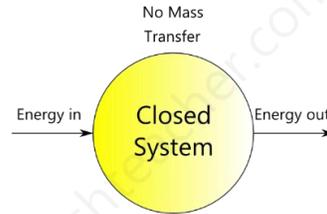
**Example of closed system:** Water heated in a closed vessel – Here only heat energy can pass in and out of the vessel.
