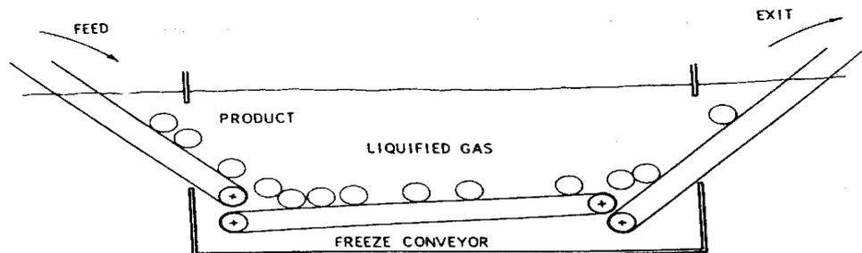
**6.11** A continuous immersion freezing system.
