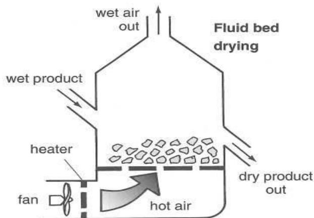
**Fig: Fluidized bed drying**
