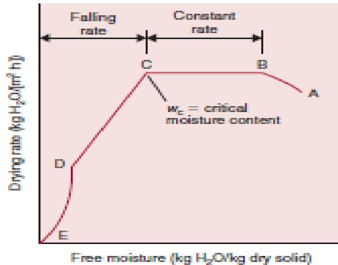
Fig: Drying Rate Curve
