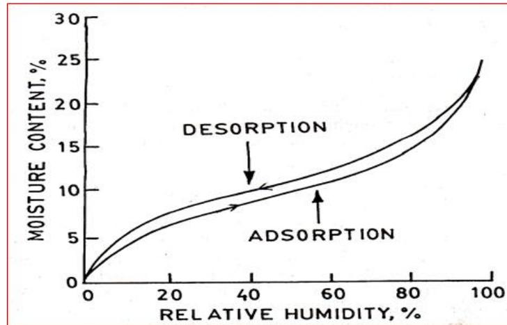
Figure: Water adsorption isotherm, Desorption isotherm and Hysteresis of moisture sorption of wheat at 35°C
