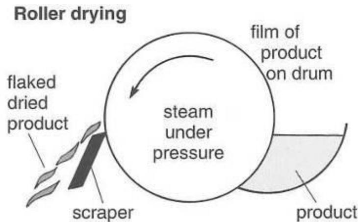
Fig: Roller drying
