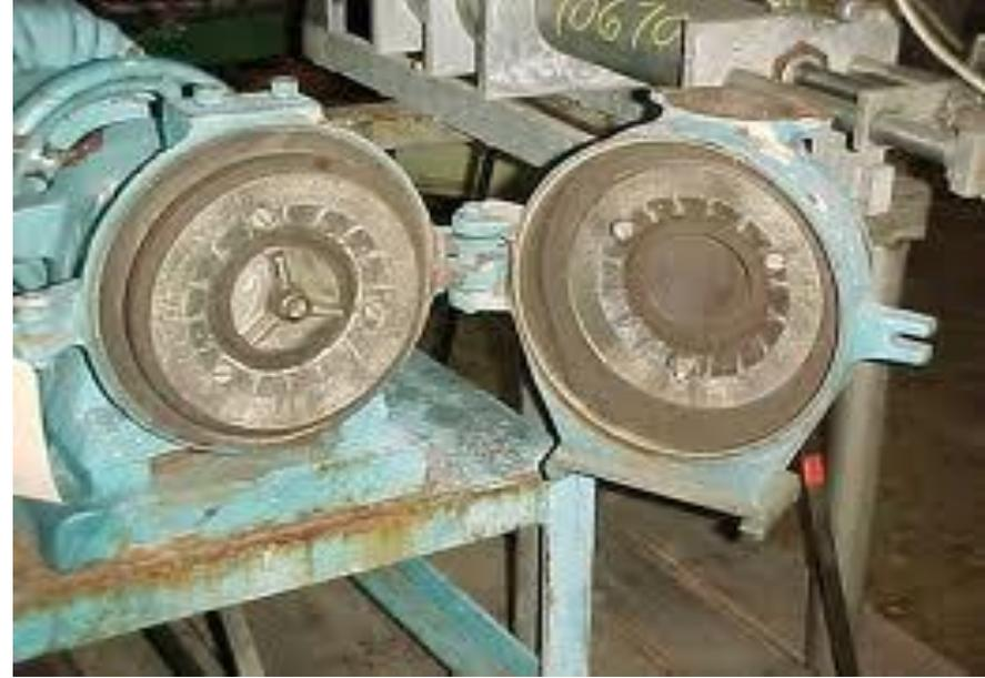
**c. Pin disc mill:** The pin disc mill carries pins on the rotating elements. In this case impact forces also play a significant part in the breakdown of particulate matter.
