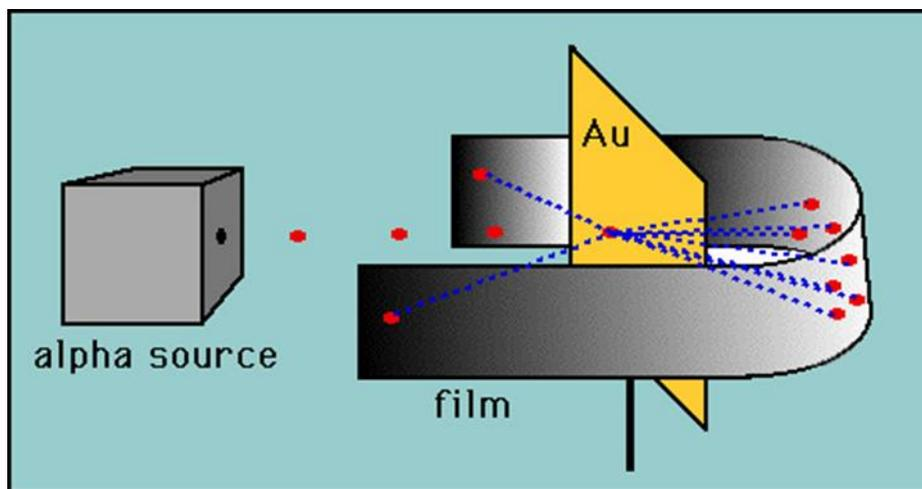
Rutherford, in his experiment, directed high energy streams of  $\alpha$ -particles from a radioactive source at a thin sheet (100 nm thickness) of gold. In order to study the deflection caused to the  $\alpha$ -particles, he placed a fluorescent zinc sulphide screen around the thin gold foil. Rutherford made certain observations that contradicted Thomson's atomic model. The observations made by
